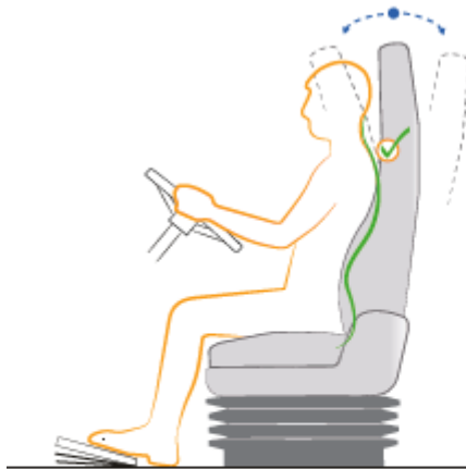
Pneumatically releasable shoulder adjustment
