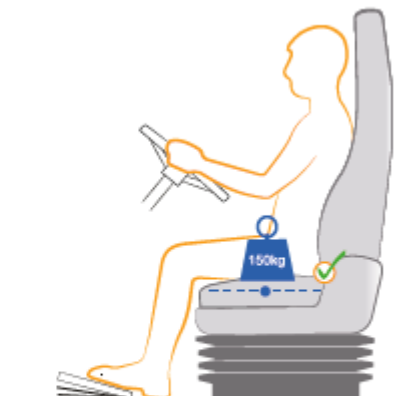
Load capacity up to 150 kg
