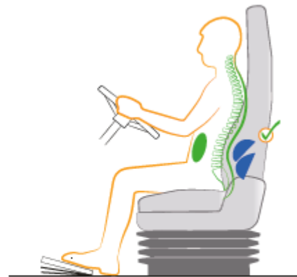
Integrated pneumatic system and lumbar support with side bolsters adaptation
