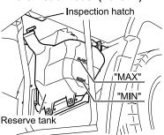
The reserve tank is located behind the front-right wheel. When the engine has cooled down, make sure that the fluid level in the reserve tank is no lower than the "MIN" line.
