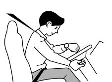
Firmly apply the parking brake. With the accelerator pedal released, turn the starter switch to the "ACC" or "LOCK" position.
