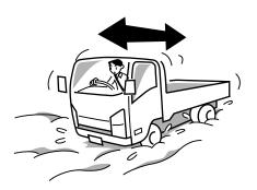
Pressing the accelerator pedal will dig the vehicle deeper into the mud and make it harder to extricate.
