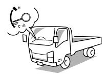
The engine is sufficiently warmed up when the needle of the engine coolant temperature gauge starts to move.
