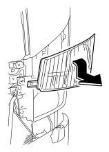
3. Tilt the turn signal light unit down toward the front of the vehicle and remove it.
