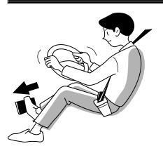
For hydraulic brake models, as the brake booster will no longer operate, brake effectiveness will be reduced. Do not panic. Press the brake pedal to reduce speed, head immediately for a safe place, stop the vehicle and perform an inspection. If the engine cannot be started, promptly have the vehicle inspected and repaired by the nearest Isuzu Dealer.
