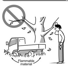
Stop the vehicle at a safe place free of flammable materials such as grass or wastepaper.
