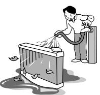
If foreign matter (insects, mud, etc.) gets stuck in the radiator's air passages, the cooling system's performance will deteriorate. Check the air passages for clogging, and remove any foreign matter using water under low pressure.
