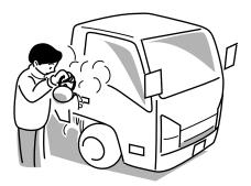
If you try to force the key into the door, you could bend it. And if you try to pull the door open with undue force, the rubber seal around the door could come unstuck or become damaged. Use warm water to melt the ice, then quickly wipe it away and open the door.
